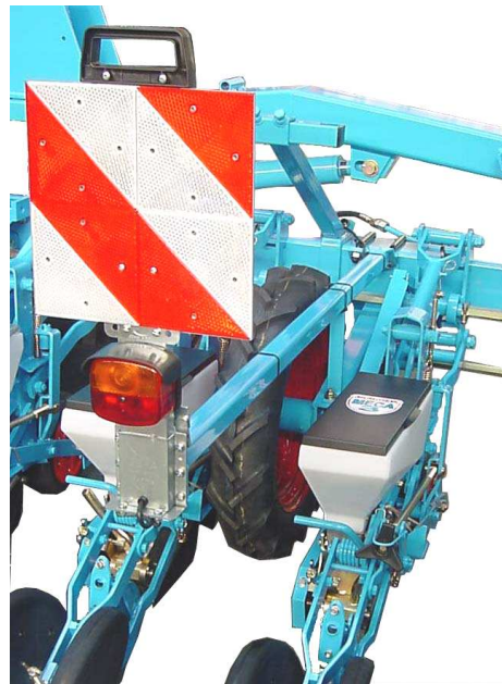
Montage du support sur MECA V4 (cas particulier fig.2) Assembly of the support bracket on the MECA V4 planter (special case fig.2) Montage des Beleuchtungshalters an der MECA V4 Sämaschine (Besonderer Fall Abb.2)
