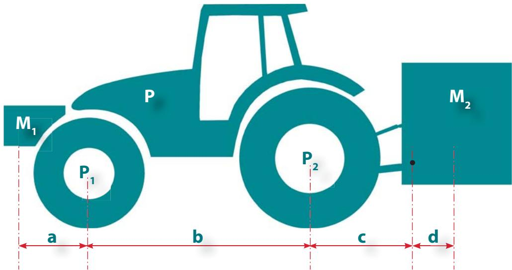
$$\textcolor{red}{\diamond} M1mini = \frac{M2 \times (c + d) - P1 \times b + (0,2 \times P \times b)}{a + b} = \dots \text{Kg}$$
